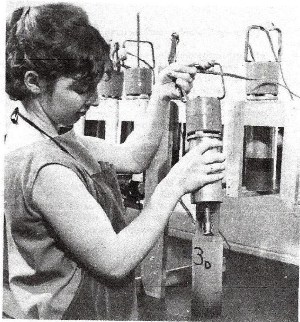
ELECTRIC MIXER is used to prepare the soil-water slurry for sampling.
